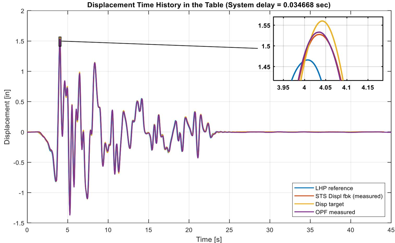
The time delay (average 34 ms) introduced by the shake table system was alleviated with an ATS compensator.
