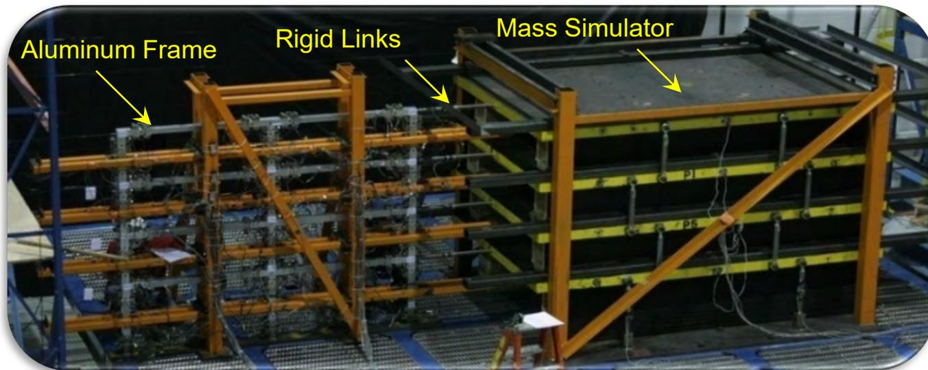
NEES Project on collapse assessment using shake table testing (**Lignos , Krawinkler and Whittaker 2011**)
