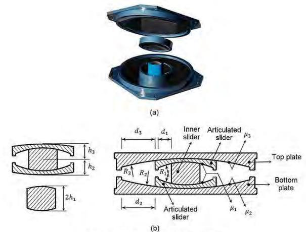
Figure 1: Triple friction pendulum bearing
