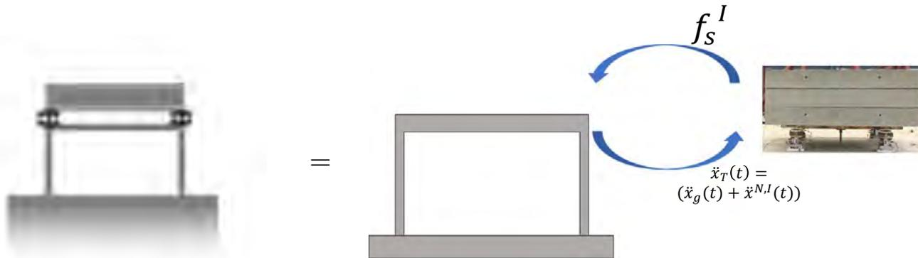
$$M^N \ddot{x}(t) + C^N \dot{x}(t) + K^N x(t) = -M^N L \ddot{x}_g(t) + f_s^I$$
